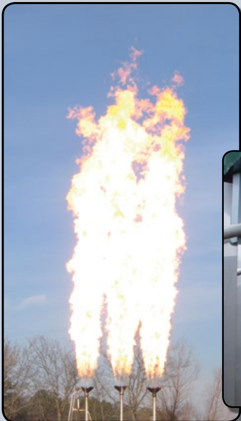
100% Xylene Testing in Zeeco's Test Facility
