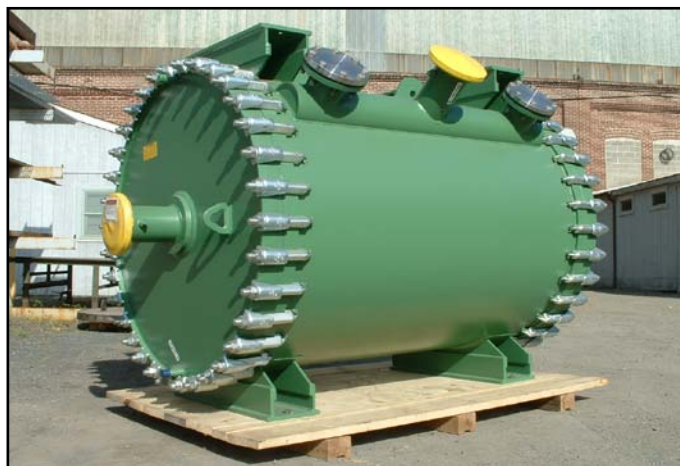
STEEL / COKE OVEN BY-PRODUCTS, Ammonia Liquor Cooler Type 1.1-H, 304/304L SS, 100" L x 60" OD 2100 ft 2 (195 m 2 )
