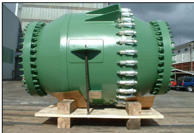
AGROCHEMICALS, Gas Cooler / Condenser Type 2-V, 316/316L SS, 75" L x 64" OD, 650 ft 2 (60 m 2 )
