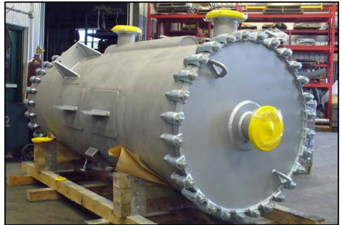
CHEMICALS, Overhead Column Condenser Type 2-V, 316/316L SS, 140" L x 50" OD, 1000 ft 2 (93 m 2 )
