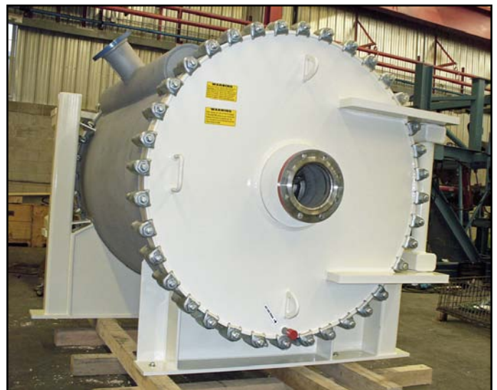
PULP & PAPER, Foul Condensate Stripping Column Preheater Type 1.1-H, 316/316 L SS, 100" L x 65" OD, 1850 ft 2 (170 m 2 )
